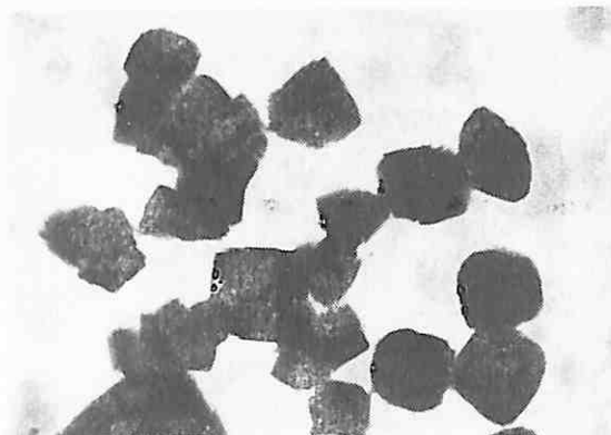
Sl. 8 — Talog dobijen reakcijom magnetski obrađenog rastvora \text{Na}_2\text{CO}_3 sa neobrađenim rastvorom \text{CaO} , povećanje 25.000 x. Fig. 8 — Sediment obtained by magnetically treated \text{Na}_2\text{CO}_3 solution reaction with untreated \text{CaO} solution, magn. 25,000 X.
