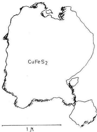
Fig. 33 — Chalcopyrite grain from K-amile xantate solution, concentration 30 mg/l. Direct magnification 31.920 x, total magnification 48.000 x.
